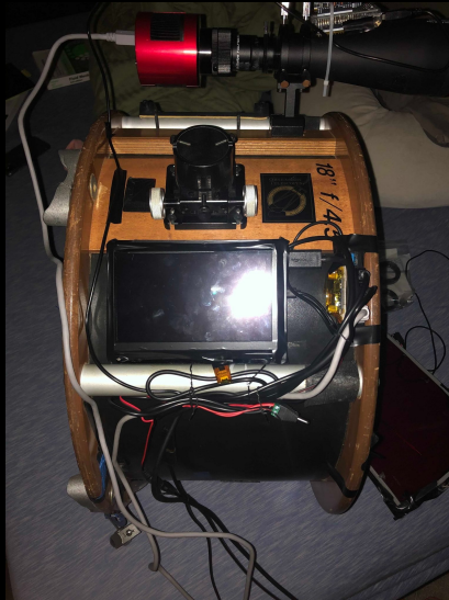
Display assembly: HDMI Monitor + Red filter + Touchscreen panel
