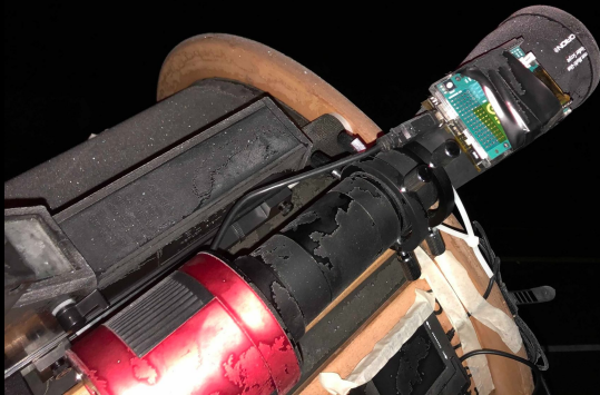
Finder scope assembly: Finder scope + CMOS Camera + Arduino with IMU Shield
